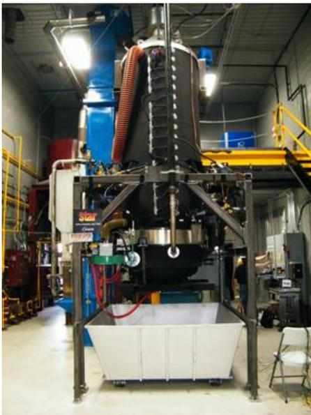
Photo 4. STAR Ex Situ Reactor (Courtesy of RESTORE).
