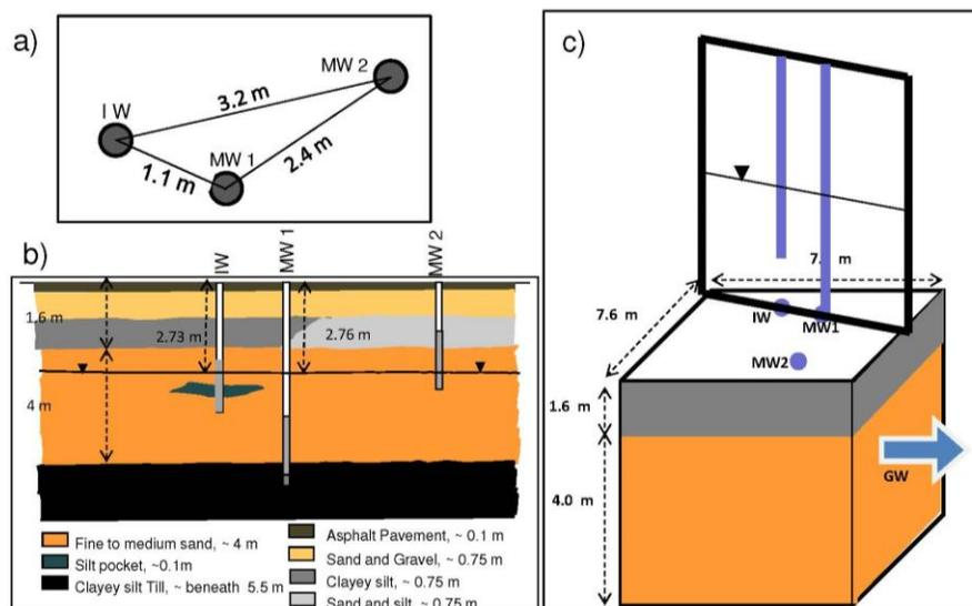
Figure 1. nZVI Transport - Model Development: (a) relative well locations at the site; (b) cross-section of study area; (c) model domain with volumetric section or plane passing through the IW-
