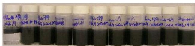
Photo 3. The effect of pH on nZVI suspension stabilized with surfactants after 24 hours of storage. The vials were prepared with nZVI (1.03g/L), surfactants and oil (ethyl caprate) in 118.8g/L of NaCl. Completely black vials indicate stable nZVI suspensions (Courtesy of Z. Wang).
