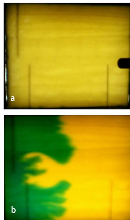
Photos 2a – 2-D CMC transport experiment before injection of CMC solution, 2b – after injection started (Courtesy P. Mondal)
