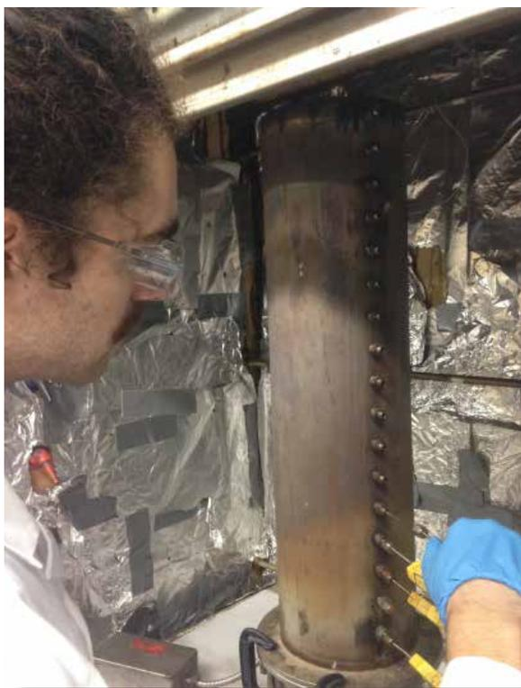
Tarek in the lab setting up his biosolids smouldering experiment. Tarek has achieved a self-sustaining smouldering reaction using biosolids with 74% moisture content at a concentration within a sand pack of 222g/kg. Photo courtesy of Tarek Rashwan.
