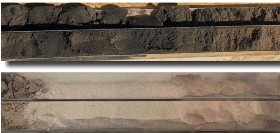
Figure 2 - Pre-STAR soil core from within the target treatment zone (top) and corresponding post-STAR soil core (bottom). Courtesy - Laura Kinsman.
