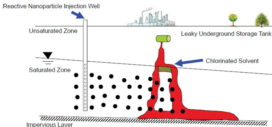
Figure 1: Field injection of nanoparticles, source: Center for Groundwater Research (CGR). 2009, courtesy of Dr. Denis O'Carroll.
